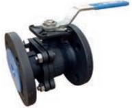
ISO 5211 for Direct Mount, Flanged **PN16 RF**, 2 Piece WCB Carbon Steel Body, Full Bore, CF8 Stainless Steel Ball, 304 Stainless Steel Stem, **TFM 1600** Seats, Graphite Packing, Firesafe to **API 607 & TA-LUFT Approved**
